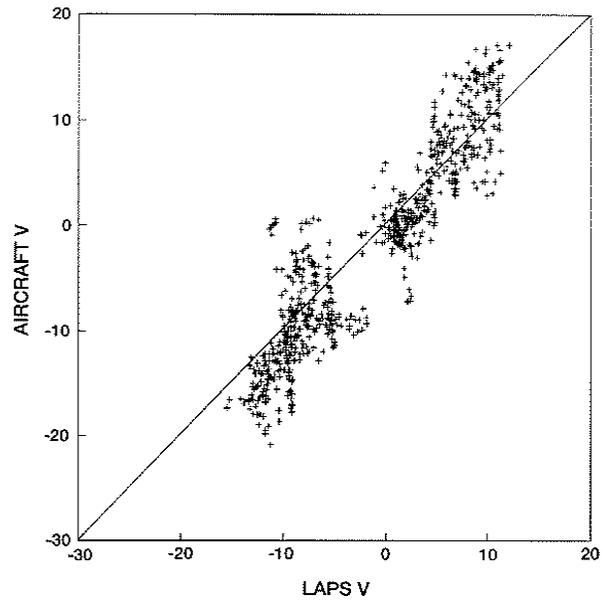
Fig. 7. Scatterplot of u wind component (a) and v wind component (b) as measured by WISP aircraft vs. the LAPS wind analysis interpolated to the aircraft location. Units are meters per second. RMS errors are  $4.0 \text{ m s}^{-1}$  and  $3.7 \text{ m s}^{-1}$ , respectively.
