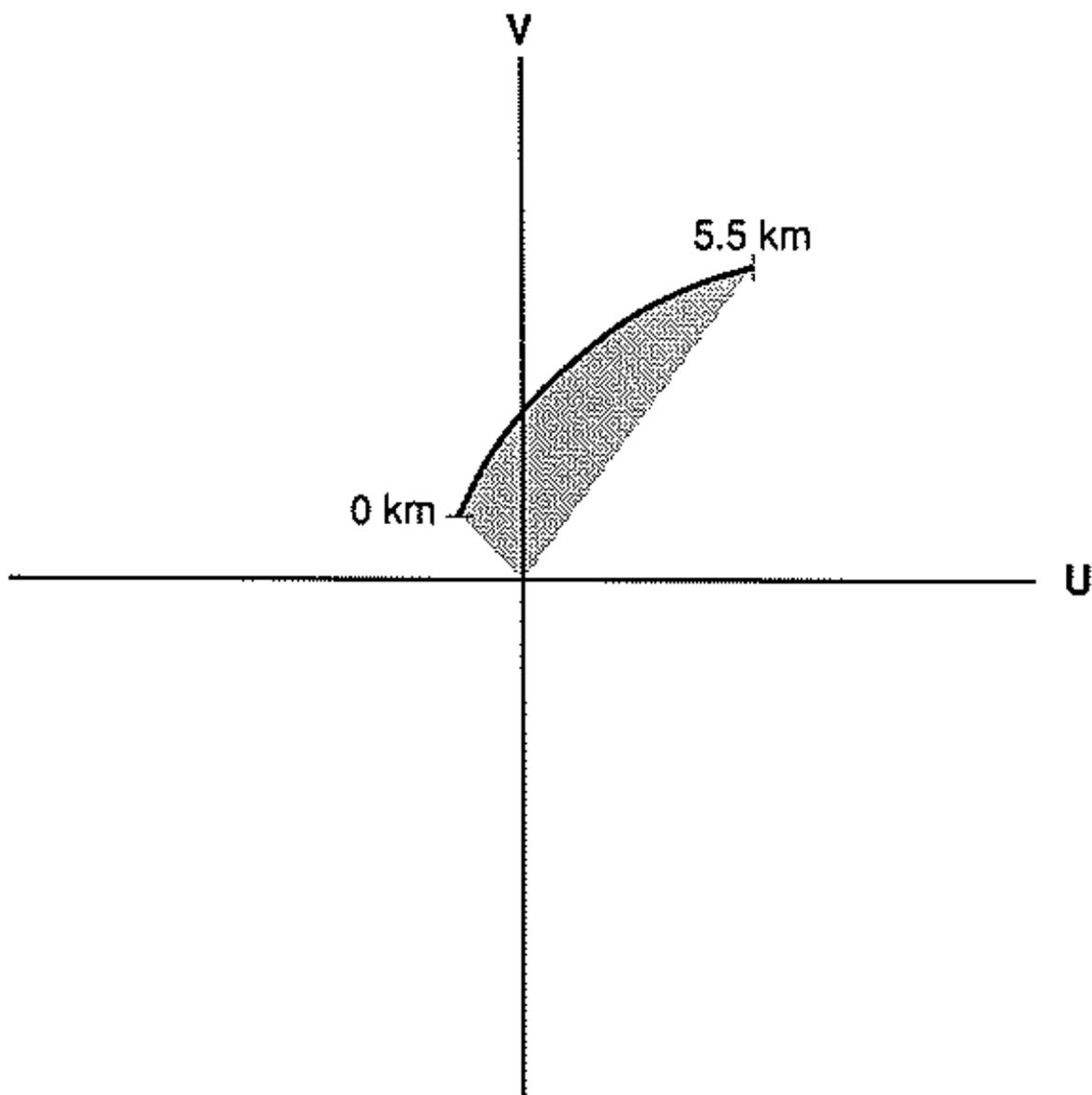
Fig. 6. The area of the hodograph swept out within a layer yields the layer mean environmental helicity. The coordinates represent the storm-relative reference frame. The shaded area in the hodograph represents the helicity in the sounding.
