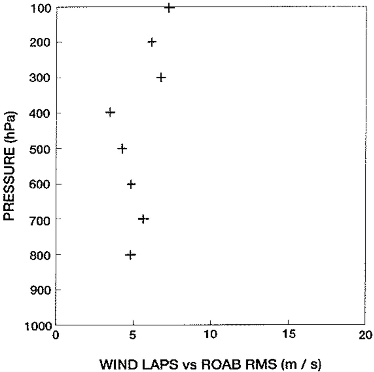
Fig. 9. RMS residuals of LAPS wind analysis compared against independent radiosonde measurements near Denver, Colorado. This represents the aggregate of soundings taken twice daily during approximately the last half of 1992. Units are  $\text{m s}^{-1}$ .
