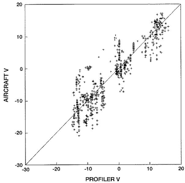
Fig. 8. Scatterplot of u wind component (a) and v wind component (b) as measured by WISP aircraft vs. a simple nearest profiler analysis. Units are meters per second. RMS errors are  $4.1 \text{ m s}^{-1}$  and  $4.0 \text{ m s}^{-1}$ , respectively.
