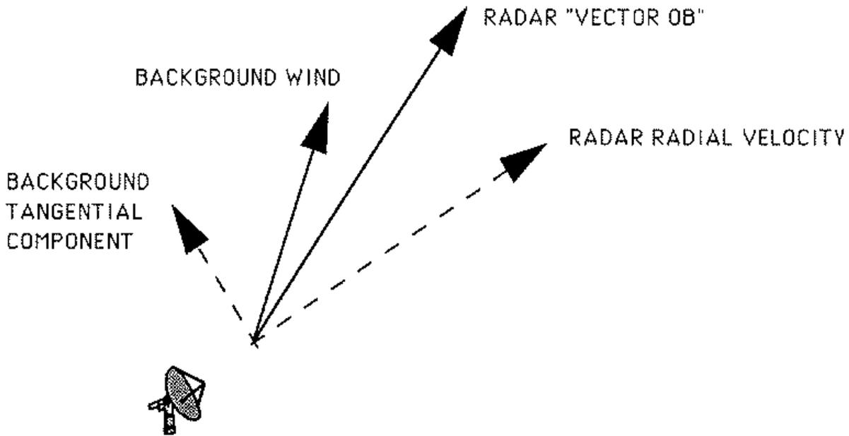
Fig. 4. Illustration of method used to combine the radial velocity from a Doppler radar with the tangential component from a background wind field. The result is a full vector wind observation.
